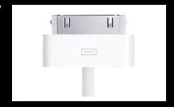
Dock Connector: One of two names for Apple's proprietary 30pin connector, which was used in all iPad, iPod, and iPhone models from 2003 through early 2012 except for iPod shuffles. Hides tiny pins for charging, data
