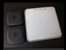
The new Apple TV is less than 1/4 the size of the original model: four Apple TVs could fit in the same space, and they're shorter, too. Matte black plastic is used on the bottom in a concave shape to minimize slippage on a flat surface, while the rest is glossy or matte plastic. A white light on the front lets you know it's on.
